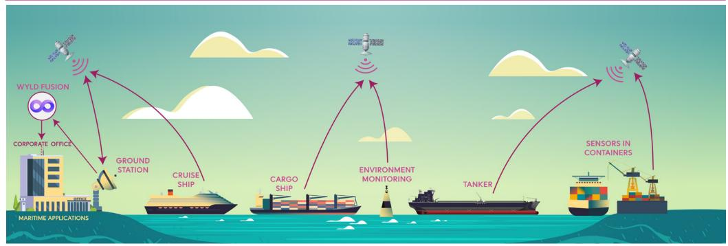
The connectivity opportunity in maritime monitoring ideally suits Wyld's direct sensor-to-satellite communication technology. Through LoRaWAN®, the low power, long range radio protocol, messages containing data points such as temperature, humidity and air quality or vibration, flow and depth can be sent directly to LEO satellites. Simple disposable batteries or rechargeables with small solar cells can last for years sending small data packets several times per day. Wyld's terminals and
